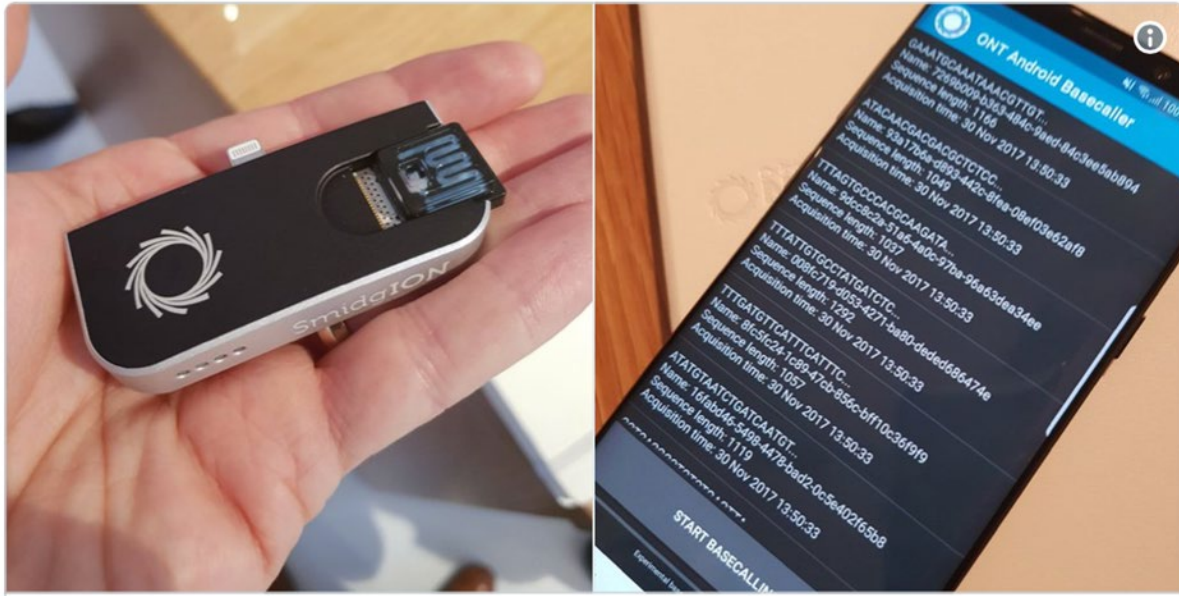
Figure 7. SmidgION and Android basecaller (Nov 2017), which is under development for portable DNA sequencing.
